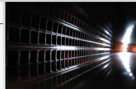
Secondary headbox installed on an existing fourdrinier
